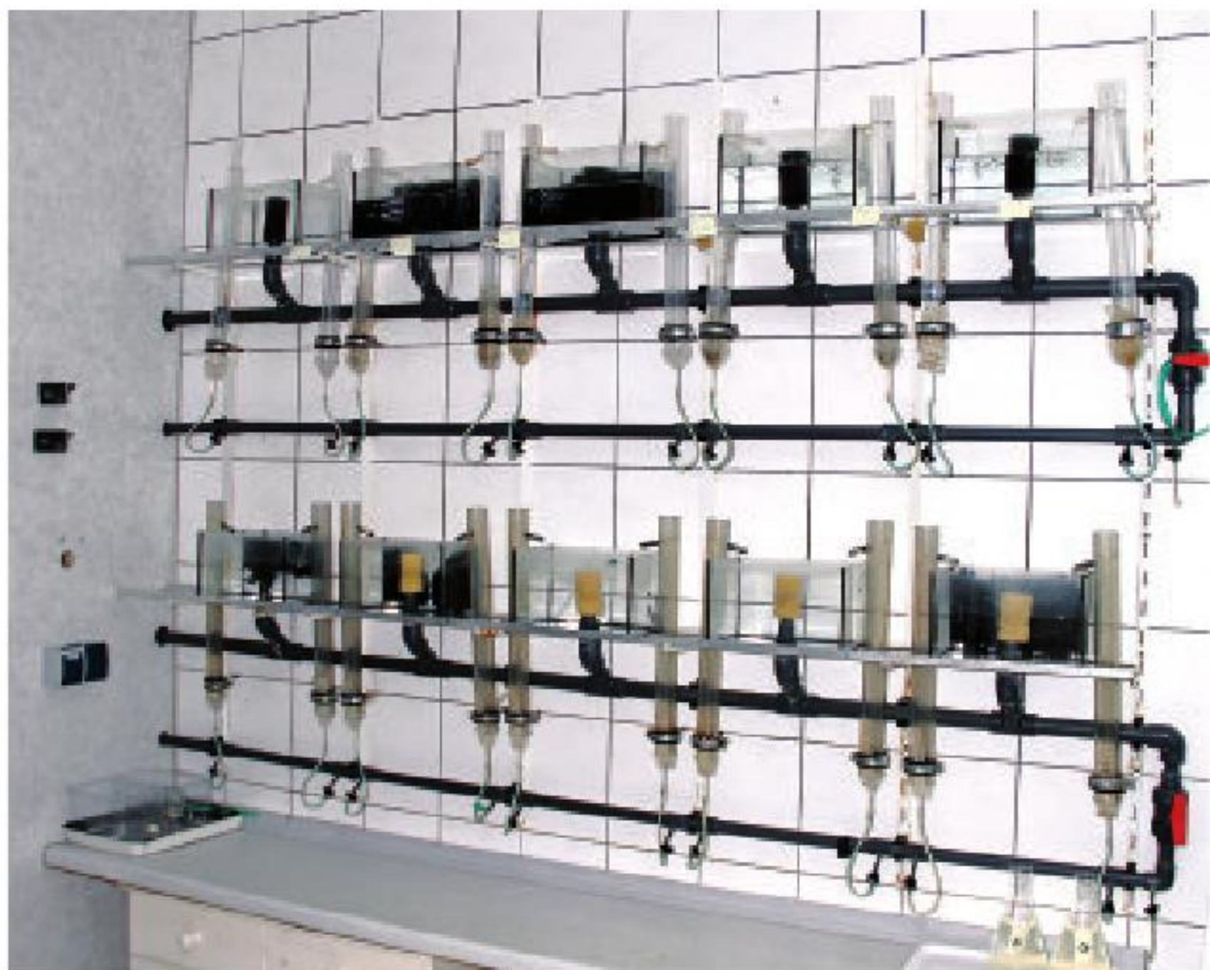
Above: This incubator unit in the laboratory is used to hatch the eggs of species that don't practice brood care. The eggs are placed in the tubes, and water is circulated via a UV unit to keep them in constant motion. Hatched larvae rise to the top and are washed into the rearing tanks, where they stay until their yolk sacs are exhausted.
